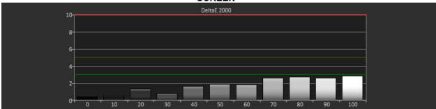
The Delta E values tell us there is no visible difference between the lens and screen measurements. All errors below the green line (3dE) cannot be seen with the naked eye. It is therefore possible to calibrate a projector from the lens and use it with the Slate .8 without further adjustments.
