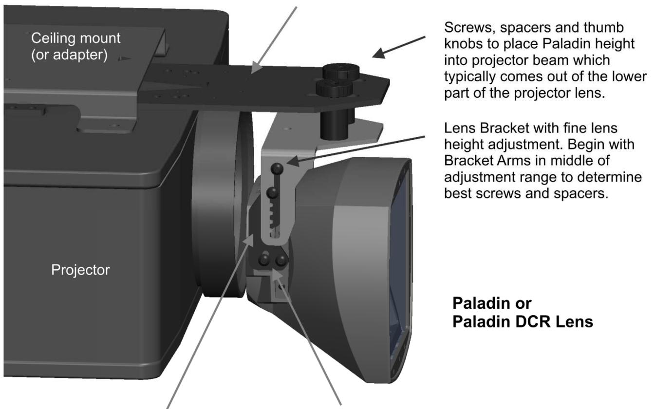
Bracket Arms. May be inverted with Lens Bracket for shelf mount with XM2 Plate under shelf-mounted projector. (lens remains in orientation shown)
